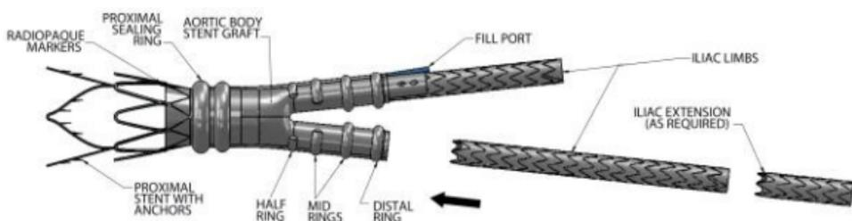
**Figure 1.** Schematic of Deployed Ovation iX Abdominal Stent Graft System
