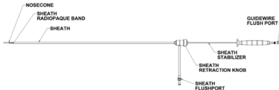
**Figure 5.** Schematic of Ovation Prime Iliac Limb/ Iliac Extension Delivery Catheter
