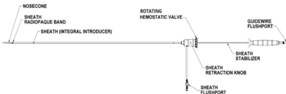
**Figure 4.** Schematic of Ovation iX Iliac Limb/ Iliac Extension Delivery Catheter
