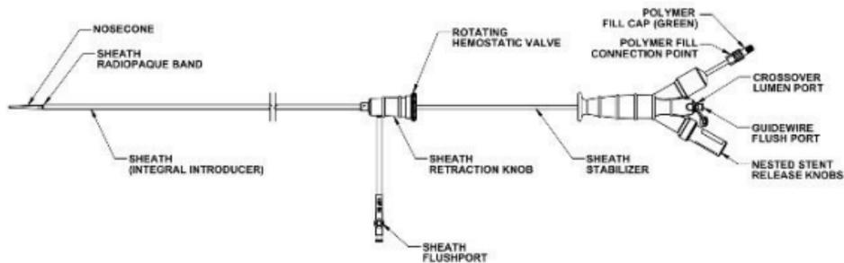
**Figure 3.** Schematic of Ovation iX Abdominal Stent Graft System Aortic Body Delivery Catheter
